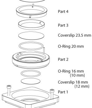
Place an O-Ring, 16.0x1.0mm {10.0x1.0mm, 22.0x1.0mm}<sup>1</sup>, on a flat surface and pick it up with Part 2.
