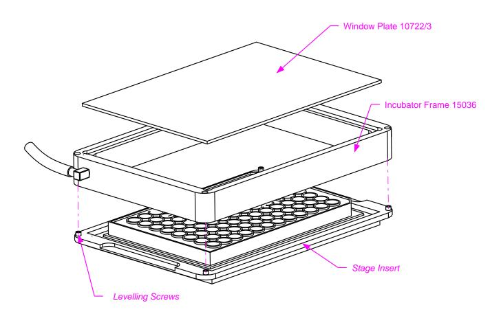
Insert a window plate into the the incubator frame 15036. Use the glass window plate 10723 if you plan to image in transillumination modes (e.g. interference contrast). Use the unbreakable polycarbonate window plate 10722 otherwise.
