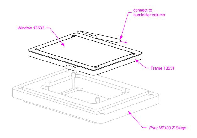
Connect the outlet of the humidifer column to one of the ports on the sides of the incubator frame using the quick connector coupling. Us as little tubing as possible, but give just enough slack so the stage can move freely. Use the port on the opposite side if re-criculation of the gas is desired or connect both ports to the humidifier column using the Y-connector for to reduce gradients in leaky setups.
