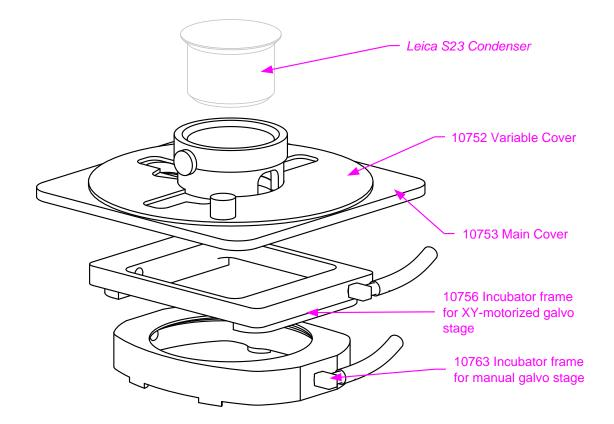
Connect the port on the side of the incubator frame 10756 or 10763 to the outlet of the humidifer column with the tubing flanges (for optimized gassing connect both ports using the supplied Yconnector piece). Place the incubator frame on the stage insert.
