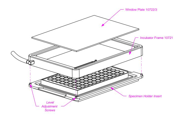
Insert a window plate into the the incubator frame 10721. Use the glass window plate 10723 if you plan to use contrast modes that require a polarization-maintaining material (e.g. interference contrast). Use the unbreakable polycarbonate window plate 10722 otherwise.
